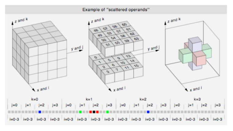
Of these seven elements of the r(i,j,k) matrix only three form an unbroken sequence in memory. Imagine
